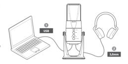
\*Notice: The USB port of computer should supply 5V power.
