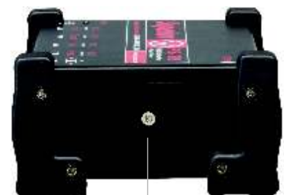
Battery compartment. Screw lock battery compartment cover. Remove the cover with a screwdriver when changing batteries.
