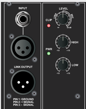
Control & Connecting Panel: Same for all active models
